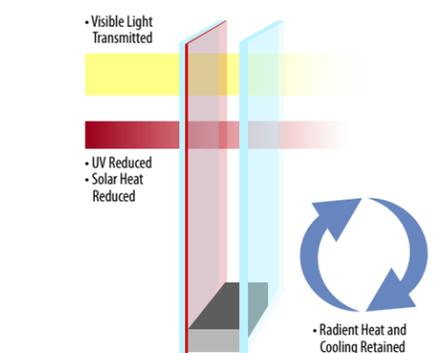
In climates where cooling is your main concern, SunSeal® Glass products are designed to reduce solar heat while still providing color-neutrality. This solar control property, combined with thermal insulating benefits, results in beautiful, natural-looking glass that helps keep air conditioning costs low.
